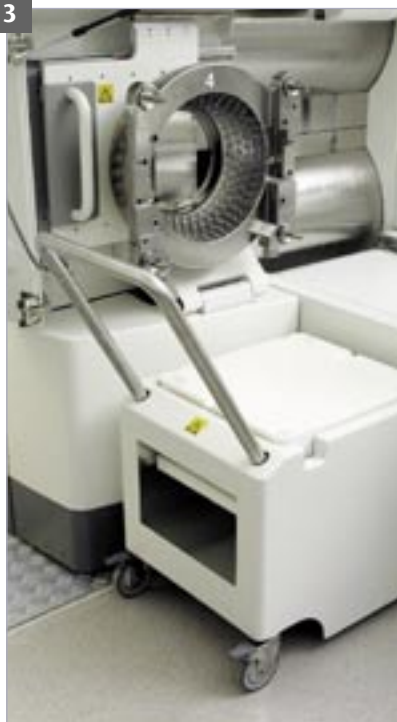
3. Sliding the helmet changer with helmet to the outer position.
