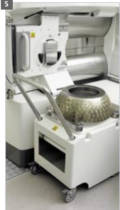
5. Releasing the helmet on the helmet trolley.
